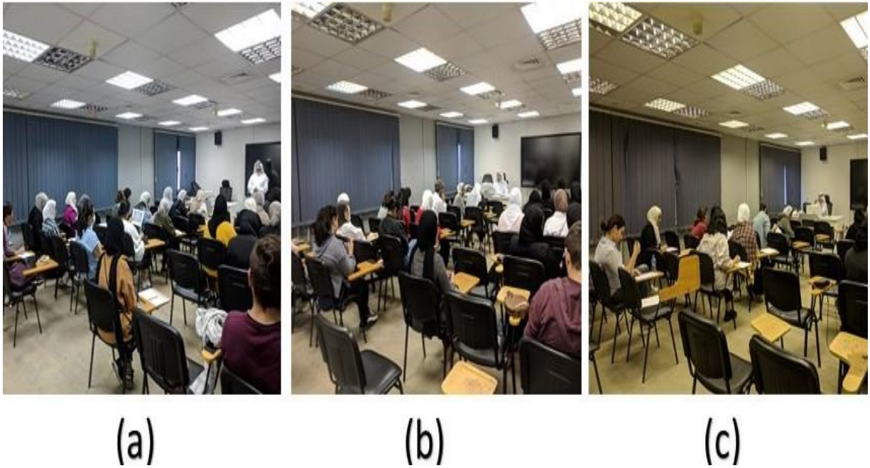
Figure 3.2: The three lighting CCT set-ups during the beginning of the lecture. A is the daylight condition 6500 K, while B is the cool white 4600 K, and C is the warm white 2700 K.
